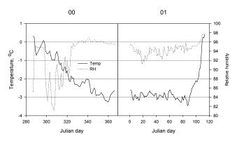
**Figure 1.** Exp. 1. Daily mean temperature and relative humidity in the Norway spruce storage box during cold storage in 2000-2001 (from Julian day 287)
