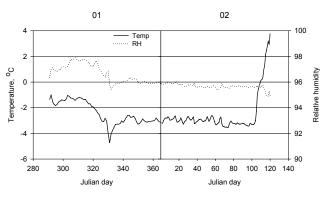
**Figure 2.** Exp. 2. Daily mean temperature and relative humidity in the Norway spruce storage box during cold storage in 2001-2002 (from Julian day 291)
